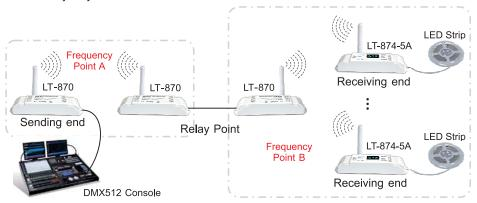
6.3 Extend the communication distance by boost antenna:
